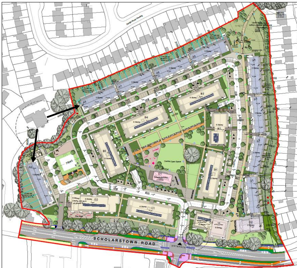
Figure 6.10 Position of Ros Mor relative to the subject site denoted, at a distance of 38m from nearest 3 storey terrace, A9 to the southwest and at 43.6m from terrace A8, due east.
